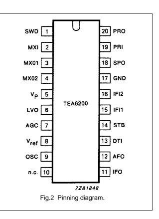
\* Pin 10 must be connected to pin 5, 8 or 17.
